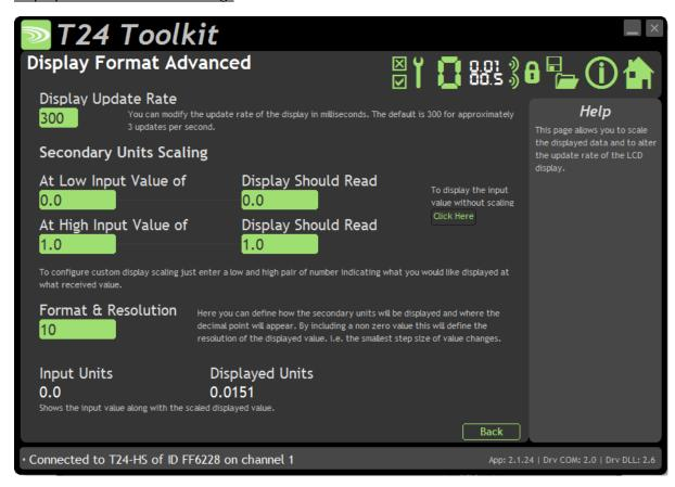
Here you can adjust the display update rate and also scale the secondary display units. This may be used, for example, to show the data from a T24-SA in tonne as the primary unit and pounds as the secondary unit.
