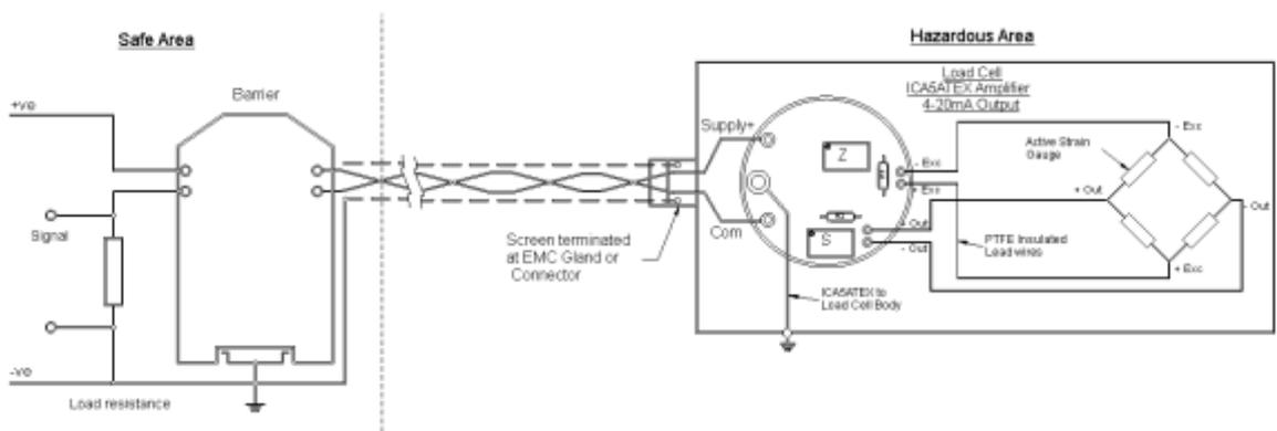
The barrier shown above limits the amount of electrical energy that can be transferred into the hazardous area, thereby preventing the ignition of a flammable atmosphere in the event of a fault condition occurring.
